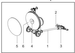
Fig. 16 Attachment of the pad
