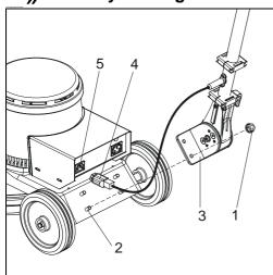
Fig. 5 Assembly of guide bar
