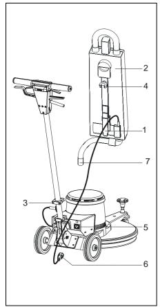
Fig. 9 Mounting the vac unit
