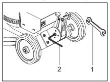
Fig. 11 Setting the swivel joint stiffness
