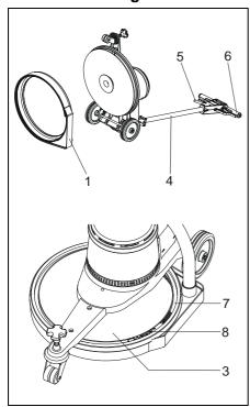
Fig. 8 Assembling the sucton ring
